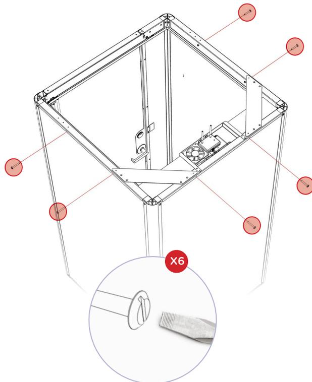
**6.** Once the roof frame is in place, use the flat head screwdriver to fully tighten all of the exterior M8 x 55 flange head bolts (16370). Bolts should be secure, but stop tightening if the wall panels begin to dimple.
