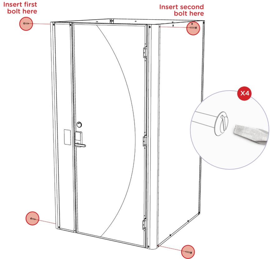
**11.** Use a flat head screwdriver to fasten the door to the base with (2) M8 x 55 flange head bolts (16370). To access the second hole, open the door by entering 8008# on the keypad. Keep the door propped open. It may be helpful to use the deadbolt to do so. Loosely tighten for now, you'll secure later.
