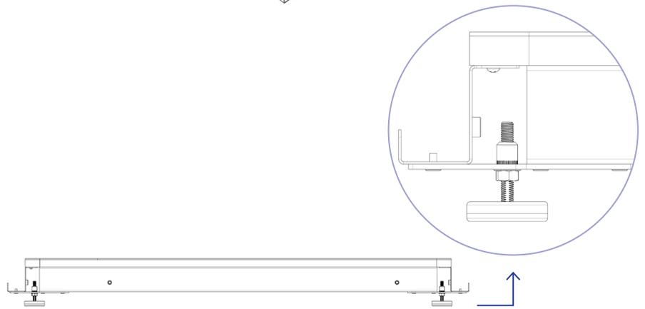
**5.** Lock each foot in place by tightening the M8 nut with an adjustable wrench until flush with the frame of the base.
