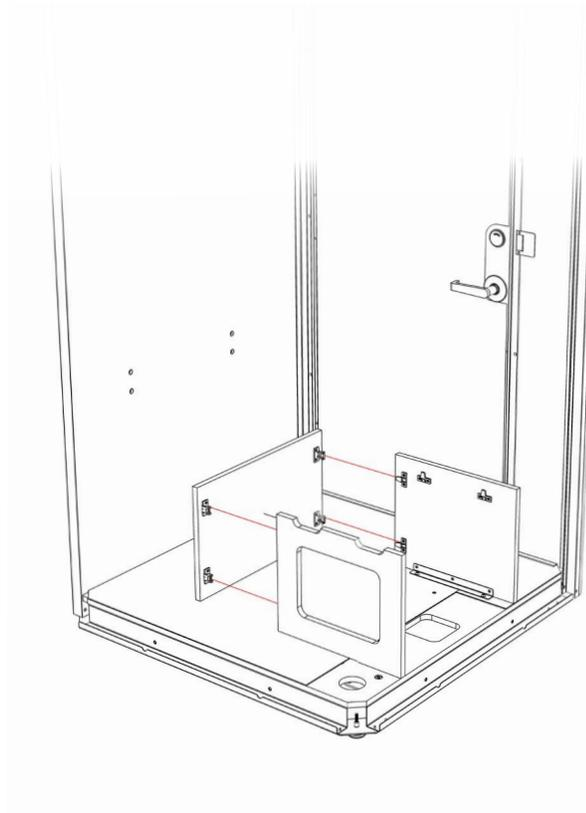
**4.** Tighten the (4) M8 x 35 button head cap screws (16840) on the seat frame right side and seat frame left side.
