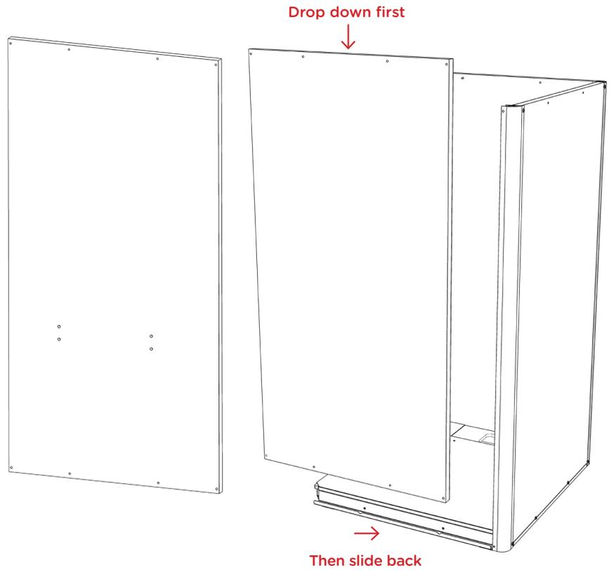
**7.** Use a flat head screwdriver to fasten the right wall panel to the base and back wall panel with (4) M8 x 55 flange head bolts (16370). Start from the upper right to stabilize the pod. Loosely tighten for now, you'll secure later.
