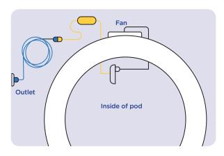
3. Inflate. Check that the fan remains unobstructed. As your pod inflates, it may need a hand to stand up until fully inflated. The pop-up will fully inflate in approximately two minutes. Pod requires power to remain inflated, but can be unplugged during off hours.
