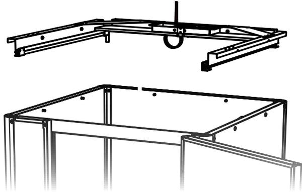
**4.** Slide the roof frame inside the top of the wall panels until the aluminum flange caps the top of the wall.
