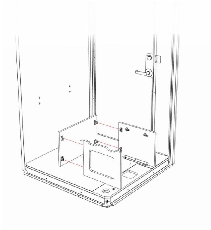
**4.** Tighten the (4) M8 x 35 button head cap screws (16840) on the seat frame right side and seat frame left side.
