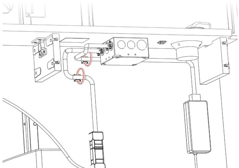
**6.** Align the plastic clips on the shelf top with the shelf frame and press down firmly.
