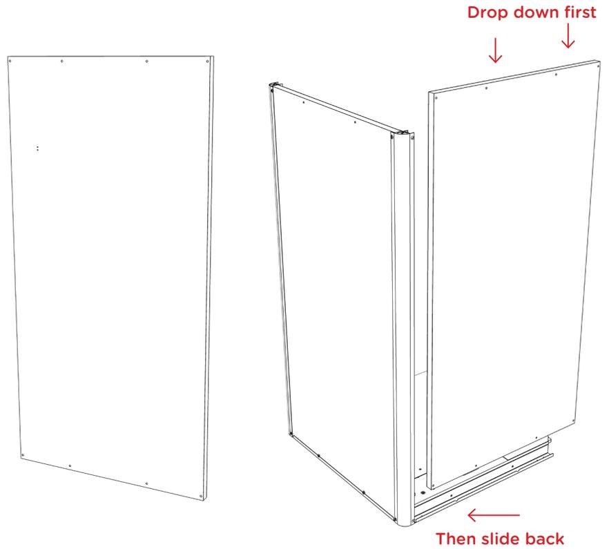
**4.** Use a flat head screwdriver to fasten the left wall panel to the foundation and back wall with (4) M8 x 55 flange head bolts (16370). Start from the top left to ensure the pod wall is stable. Loosely tighten for now, you'll secure later.
