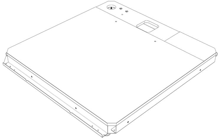
**4.** Adjust leveling feet by rotating them clockwise by hand until they extend an inch beyond the caster wheels and make contact with the floor. Make sure the base is stable.
