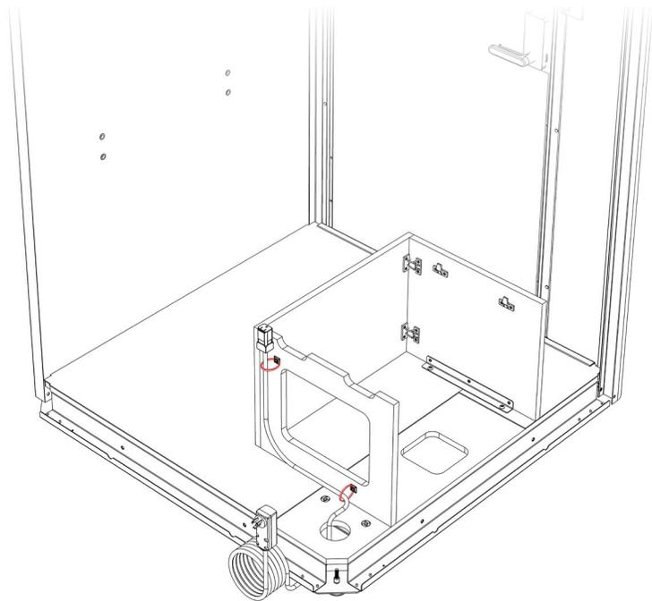
**6.** Place the seatback on its side. Use a Phillips head screwdriver and (2) 1/4" x 2" Phillips pan head screws to fasten the seatback to the seat base.
