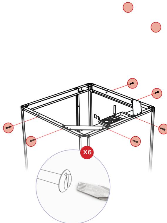
**6.** Once the roof frame is in place, use the flat head screwdriver to fully tighten all of the exterior M8 x 55 flange head bolts (16370). Bolts should be secure, but stop tightening if the wall panels begin to dimple.
