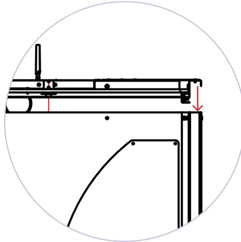
**5.** Use a flat head screwdriver to secure the roof frame to the left back and right walls with (6) M8 x 55 flange head bolts (16370). Loosely tighten as the bolts will be fully secured in the next step.
